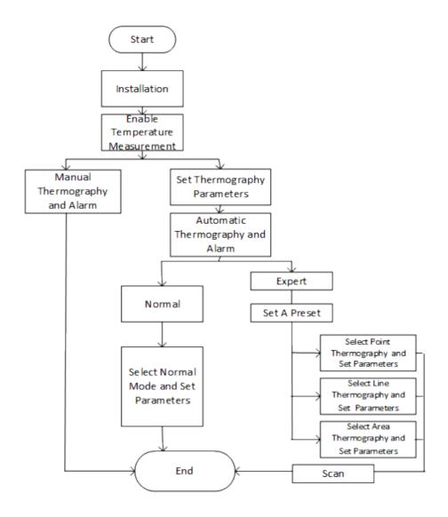
Figure 3-1 Thermography Configuration Flow Chart
